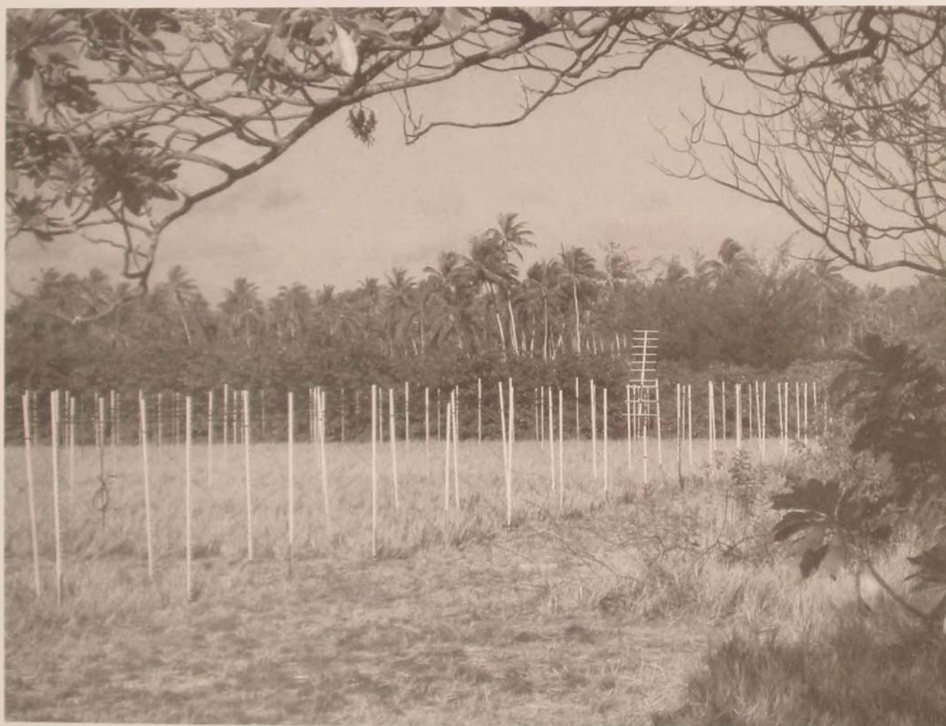
Ionospheric forecasts improve war-fighter communication efficiency. The Scintillation Network Decision Aid antenna, located on Kiritimati Island (Christmas Island), Republic of Kiribati, monitors geostationary satellite communication signals to determine the effects of ionospheric turbulence. (US Air Force photo)
